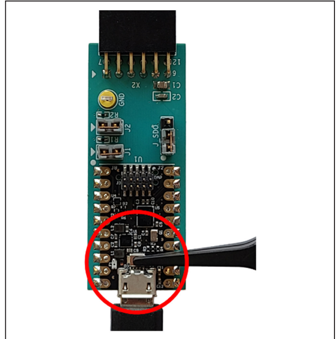
Figure 8. Enter Maintenance Mode on the MAX32625PICO.
