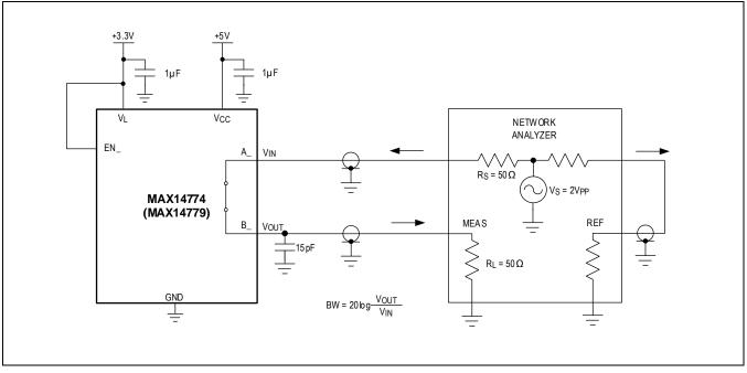
Figure 8. Frequency Response Measurement
