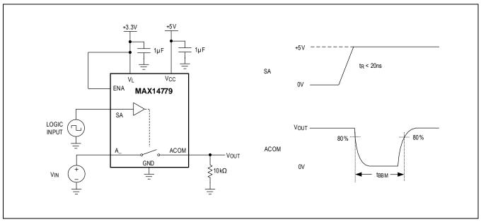
Figure 5. Break Before Make Time Measurement
