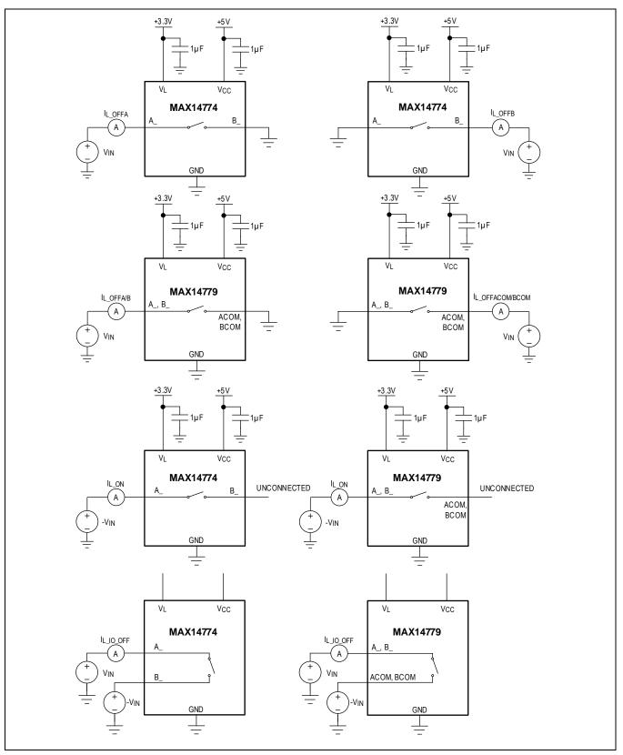
Figure 2. Leakage Current Measurements
