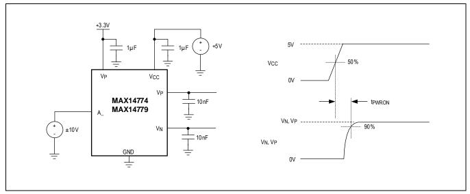
Figure 3. Power-Up Time Measurement
