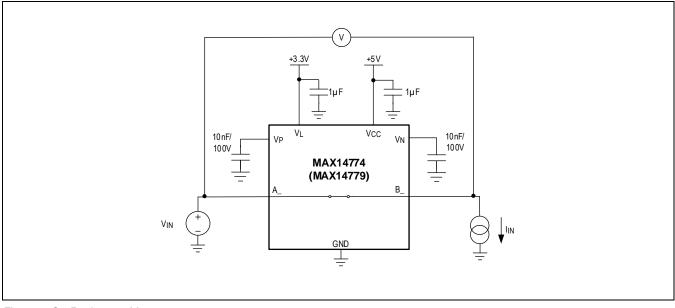
Figure 1. On-Resistance Measurement
