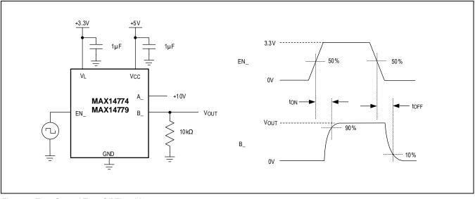
Figure 4. Turn-On and Turn-Off Time Measurement
