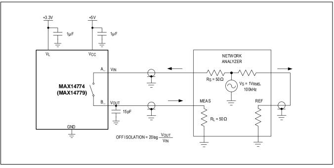
Figure 6. Off Isolation Measurement
