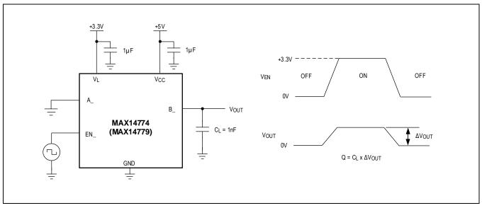
Figure 9. Charge Injection Measurement
