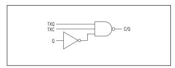
Figure 9. Equivalent C/Q Logic
