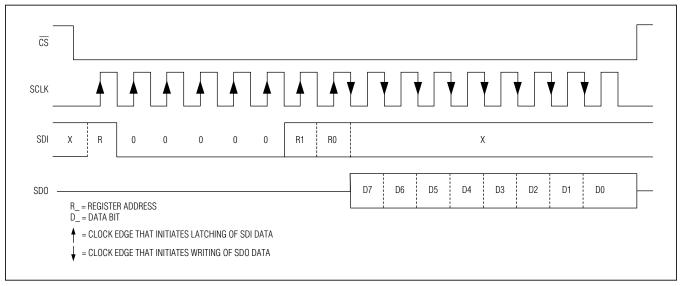
Figure 12. SPI Read Cycle
