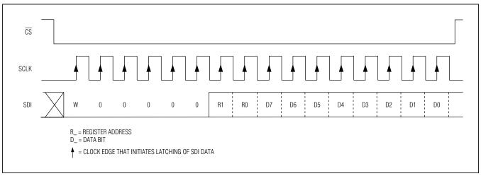
Figure 11. SPI Write Cycle
