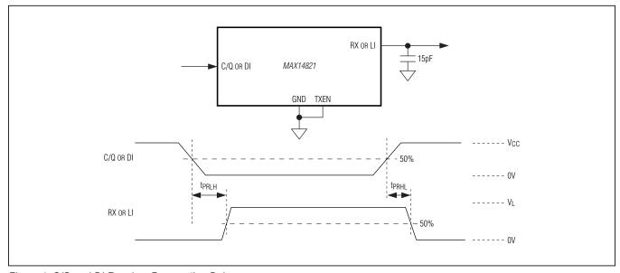
Figure 4. C/Q and DI Receiver Propagation Delays
