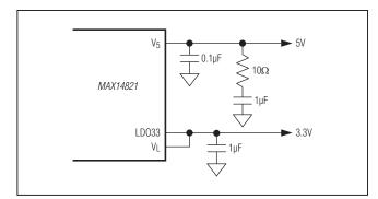
Figure 7. V<sub>5</sub> Compensation Network
