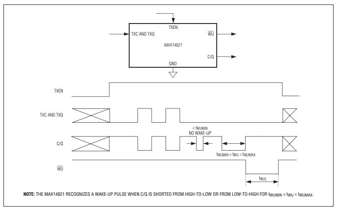
Figure 5. Wake-Up Detection Timing
