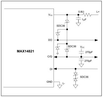
Figure 14. MAX14821 Operating Circuit with TVS Protection
