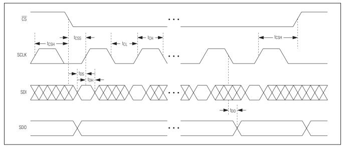
Figure 6. SPI Timing Diagram
