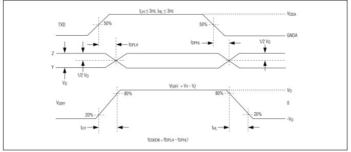
Figure 3. Driver Propagation Delays
