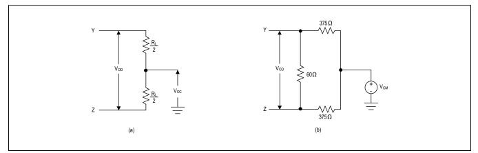
Figure 1. Driver DC Test Load
