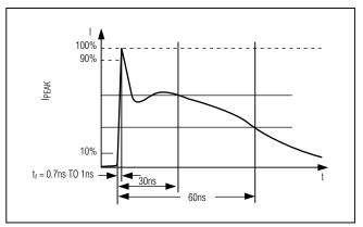
Figure 14. IEC 61000-4-2 ESD Generator Current Waveform
