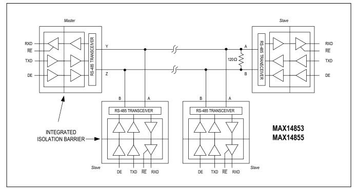
Figure 9. Typical Isolated Full-Duplex RS-485/RS-422 Application
