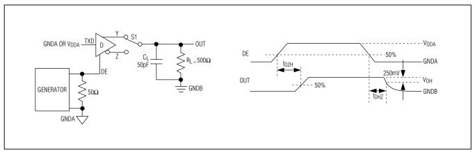
Figure 4. Driver Enable and Disable Times ( $t_{DZH}$ ,  $t_{DHZ}$ )
