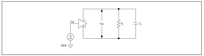
Figure 2. Driver Timing Test Circuit
