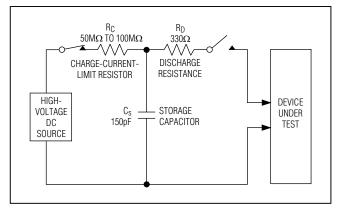
Figure 13. IEC 61000-4-2 ESD Test Model
