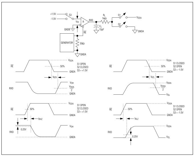
Figure 8. Receiver Enable and Disable Times
