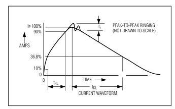
Figure 12. Human Body Current Waveform
