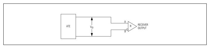
Figure 6. Receiver Propagation Delay Test Circuit
