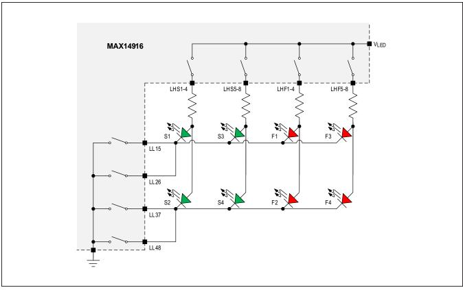
Figure 9a. LED Matrix Scheme for Quad Configuration
