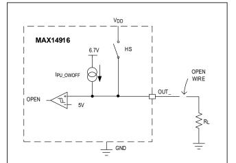
Figure 5. Open Wire Detection Scheme
