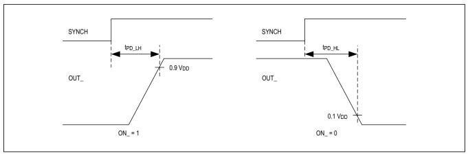
Figure 2. Propagation Delay Timing Characteristics
