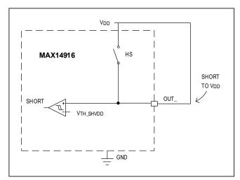
Figure 6. Short to V<sub>DD</sub> Detection Scheme
