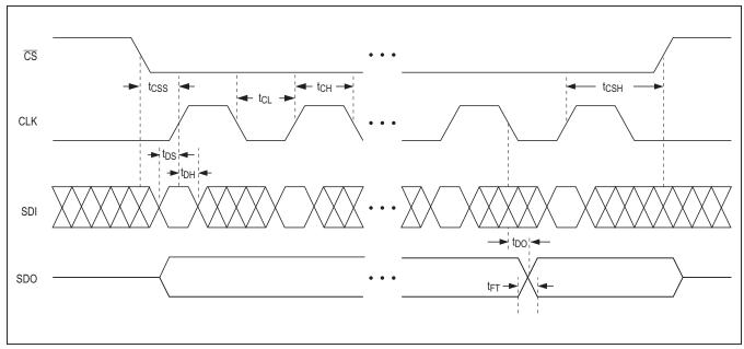
Figure 1. SPI Timing Diagram.
