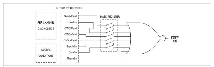
Figure 8. FAULT Signaling Scheme
