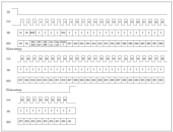
Figure 15. Addressed SPI Burst Read Command
