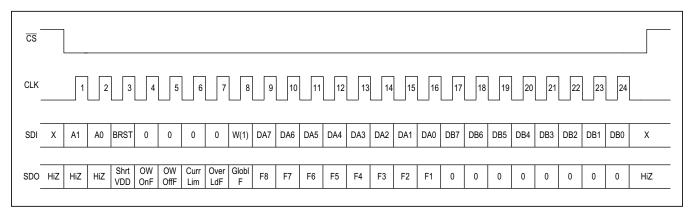
Figure 12. Addressed SPI Two Byte Write Command
