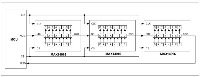
Figure 17. Daisy-Chaining Diagram of Three MAX14916
