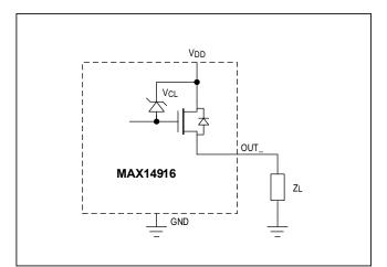
Figure 22. Inductive Load Clamping Scheme
