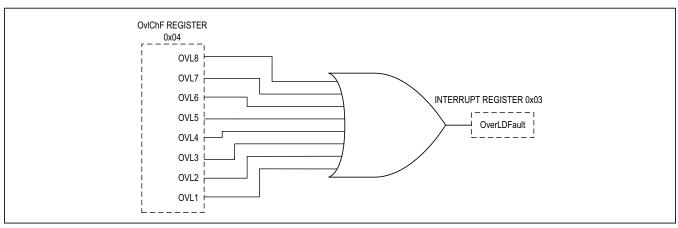
Figure 7. Overload Interrupt Diagnostic Scheme
