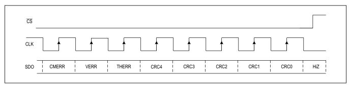
Figure 21. FCS Byte Sent by the MAX14916 to SPI Master in Daisy-Chain Mode
