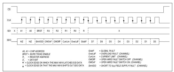
Figure 10. Addressed SPI Single Read Command
