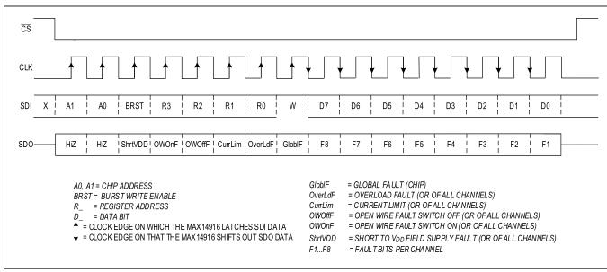
Figure 11. Addressed SPI Single Cycle Write Command
