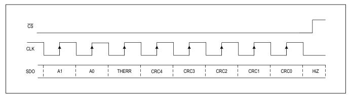
Figure 20. FCS Byte Sent by the MAX14916 to SPI Master (SPI Addressed Mode)
