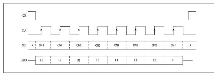
Figure 18. Single Daisy-Chain SPI Command
