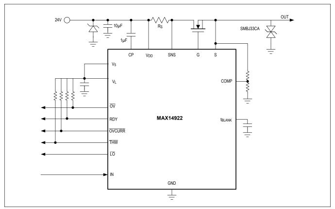
Figure 3. Transient EMC Protection Scheme
