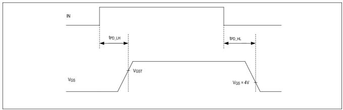
Figure 1. IN to G Propagation Times
