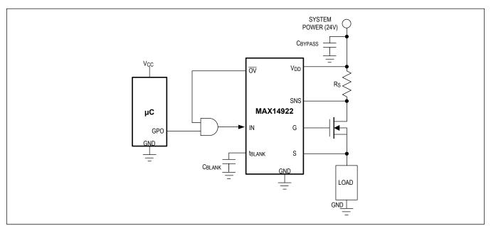
Figure 2. High Supply Shut-off Application
