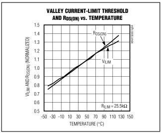
Figure 4. Current-Limit Trip Point and V<sub>RDS(ON)</sub> vs. Temperature
