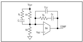
Figure 7a. Type III Compensation Network
