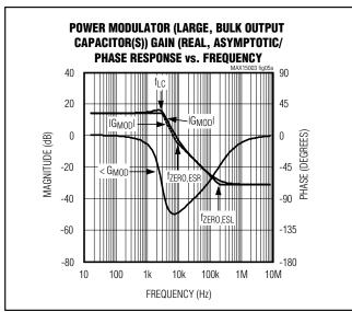
Figure 5a. Power Modulator Gain and Phase Response (Large, Bulk COUT)
