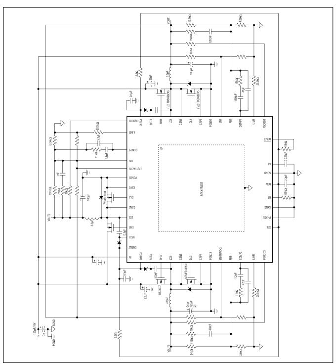
Figure 8. Coincident Triple Tracker with Lossless Current Sense
