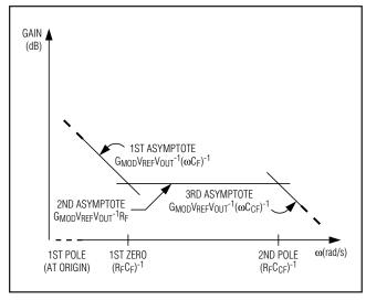
Figure 6b. Type II Compensation Network Response
