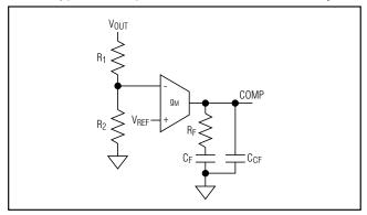
Figure 6a. Type II Compensation Network
