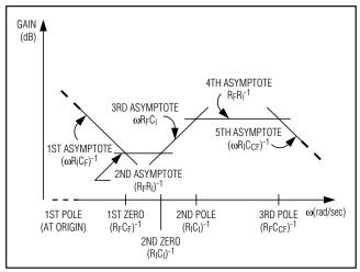
Figure 7b. Type III Compensation Network Response
