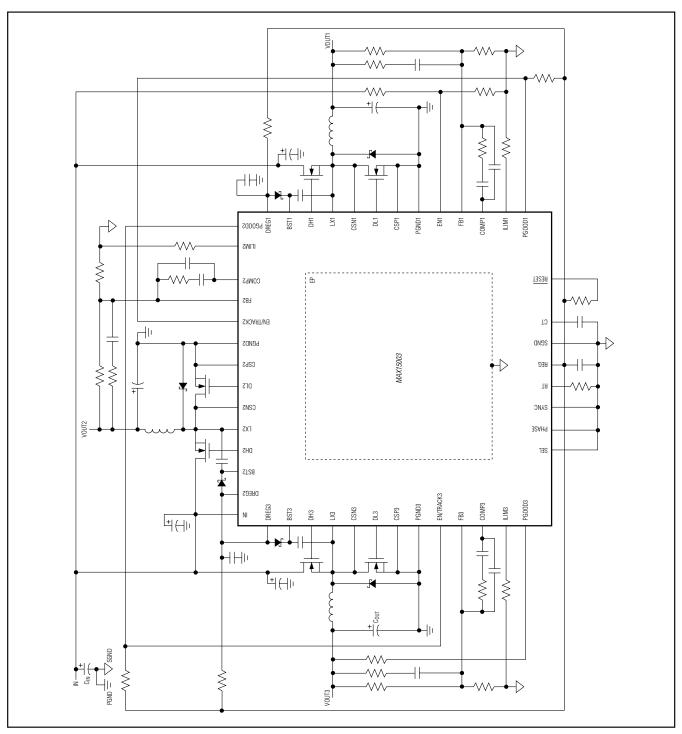
Figure 9. Triple Sequencer with Lossless Current Sense
