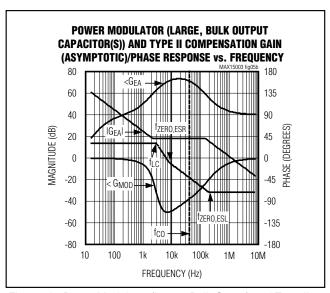
Figure 5b. Power Modulator (Large, Bulk COUT) and Type II Compensator Responses
