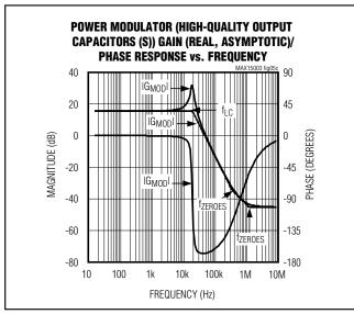
Figure 5c. Power Modulator Gain and Phase Response (High-Quality COUT)
