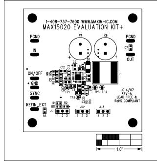
Figure 2. MAX15020 EV Kit Component Placement Guide— Component Side
