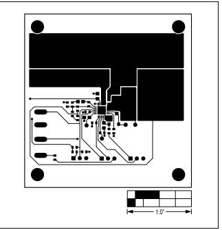
Figure 3. MAX15020 EV Kit PCB Layout—Component Side
