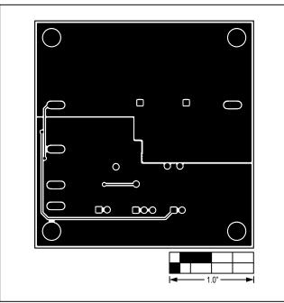
Figure 4. MAX15020 EV Kit PCB Layout—GND Layer 2
