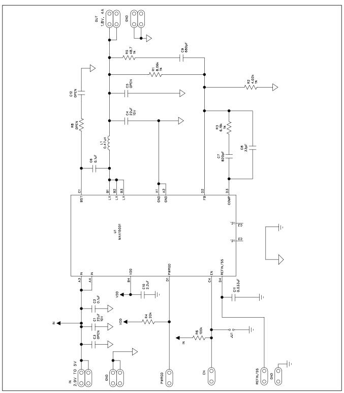
Figure 1. MAX15051 EV Kit Schematic
