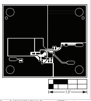
Figure 3. MAX15051 EV Kit Component PCB Layout—Component Side
