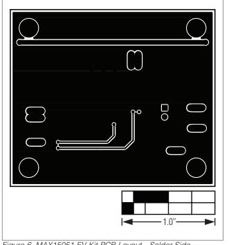
Figure 6. MAX15051 EV Kit PCB Layout—Solder Side
