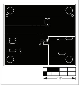
Figure 4. MAX15051 EV Kit PCB Layout—Inner Layer 2
