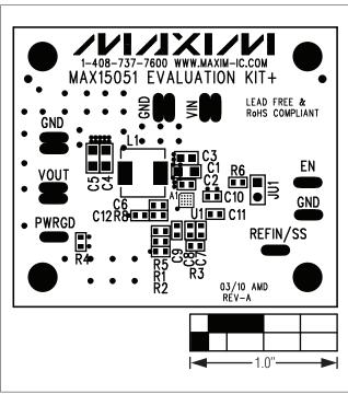
Figure 2. MAX15051 EV Kit Component Placement Guide— Component Side
