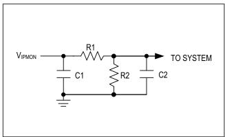
Figure 2. External RC Network to Adjust VIPMON
