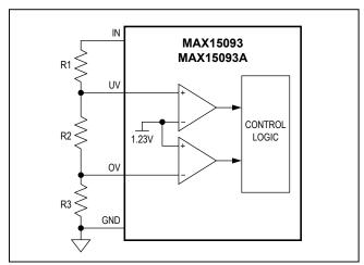
Figure 1. Undervoltage/Overvoltage-Threshold Setting
