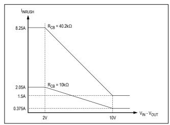
Figure 2. Startup Inrush Current Foldback Characteristics
