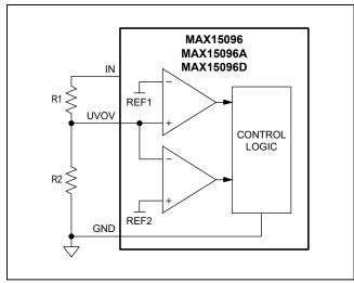
Figure 1. Undervoltage/Overvoltage Threshold Setting
