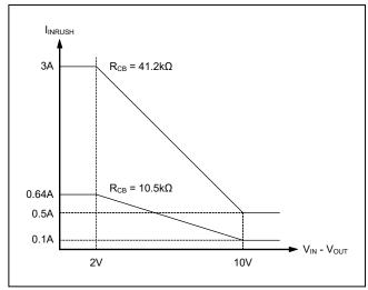
Figure 2. Startup Inrush Current Foldback Characteristics
