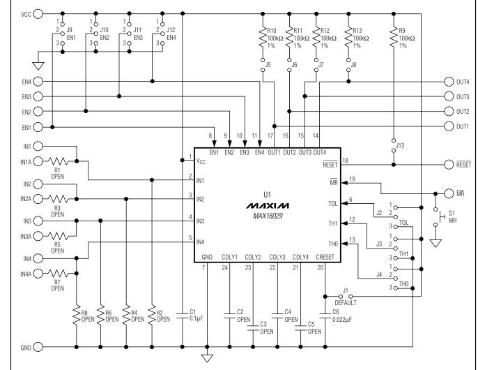
Figure 1. MAX16029EV Kit Schematic
