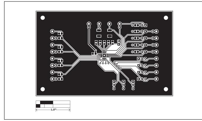
Figure 3. MAX16029EV Kit PCB Layout—Component Side
