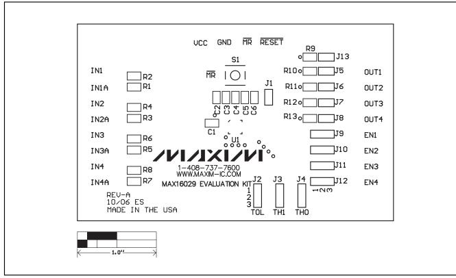
Figure 2. MAX16029EV Kit Component Placement Guide—Components Side
