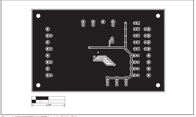
Figure 4. MAX16029EV Kit PCB Layout—Solder Side
