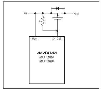
Figure 20. Connection for a p-Channel Series-Pass MOSFET
