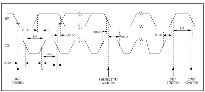
Figure 1. I<sup>2</sup>C/SMBus Timing Diagram
