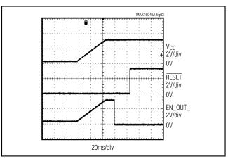
Figure 3. RESET and EN\_OUT\_ During Power-Up, EN\_OUT\_ Is in Open-Drain Active-Low Configuration
