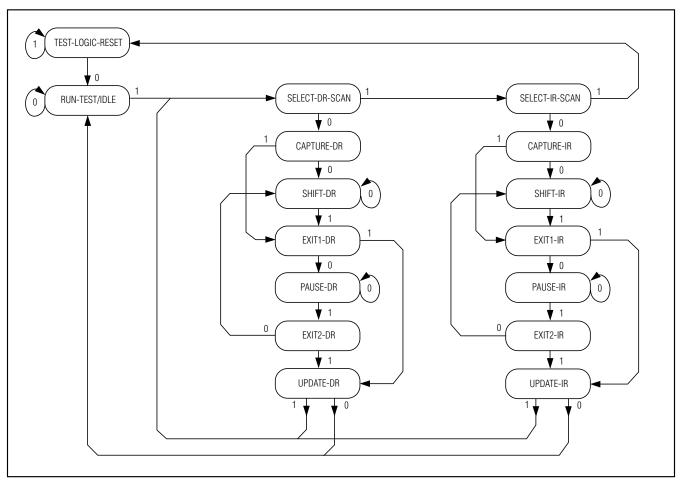
Figure 14. TAP Controller State Diagram
