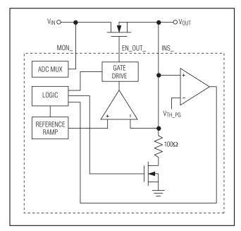
Figure 19. Closed-Loop Tracking
