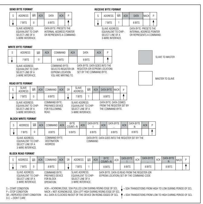
Figure 12. I<sup>2</sup>C/SMBus Protocols
