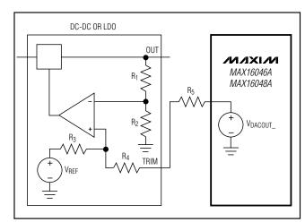
Figure 17. Connections for Margining Using Trim Input Method
