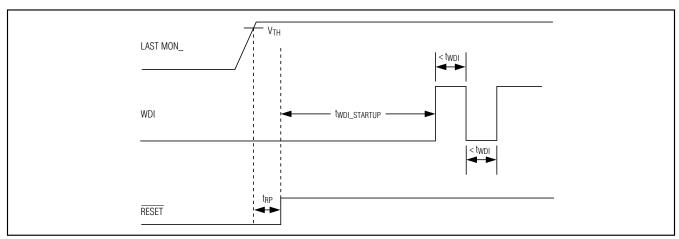
Figure 6. Normal Watchdog Startup Sequence
