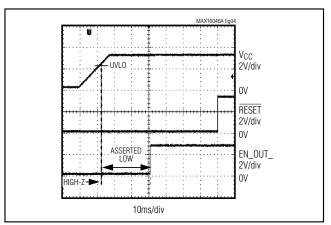
Figure 4. RESET and EN\_OUT\_ During Power-Up, EN\_OUT\_ Is in Push-Pull Active-High Configuration
