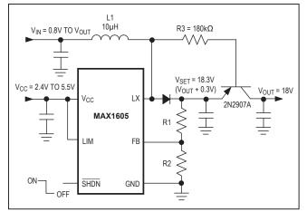
Figure 5. Output Disconnected in Shutdown
