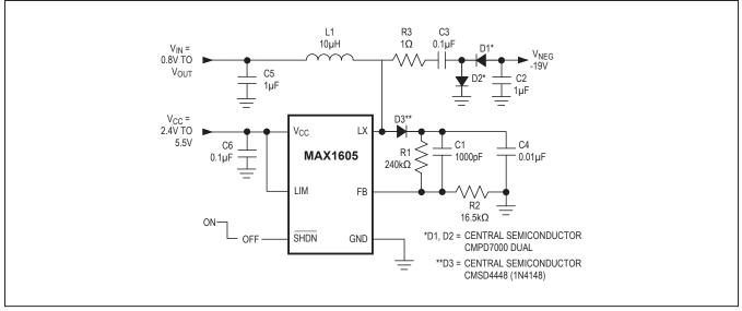
Figure 4. Negative Voltage for LCD Bias
