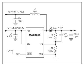
Figure 3. Typical Application Circuit
