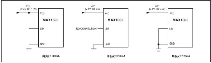
Figure 2. Setting the Peak Inductor Current Limit
