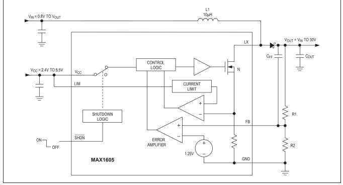
Figure 1. Functional Diagram
