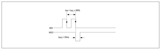
Figure 3. Fast Watchdog Fault Timing Characteristics
