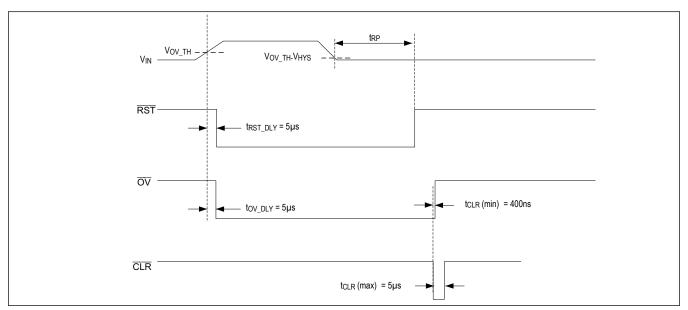
Figure 2. Clear Input Timing Diagram
