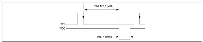
Figure 4. Slow Watchdog Timing Characteristics
