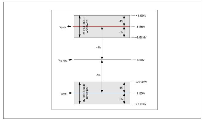
Figure 6. Undervoltage/Overvoltage Threshold Accuracy
