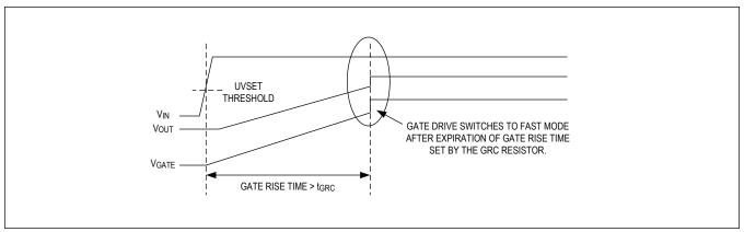
Figure 6. Gate Voltage Slow to Fast-Mode Transition
