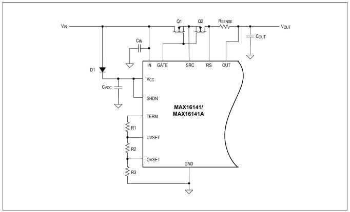
Figure 2. UVSET and OVSET Threshold Setting
