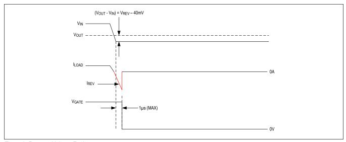
Figure 3. Reverse-Voltage Fault
