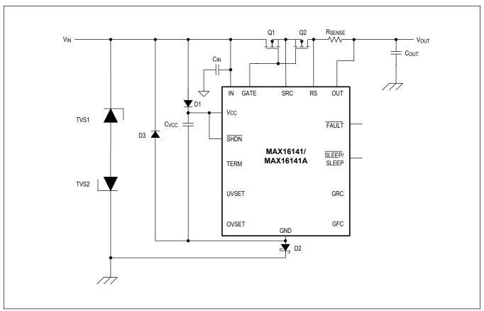
Figure 4. Recommended Reverse-Voltage Protection Circuit
