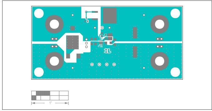
Figure 3. MAX16173 EV Kit PCB Layout—Component Side
