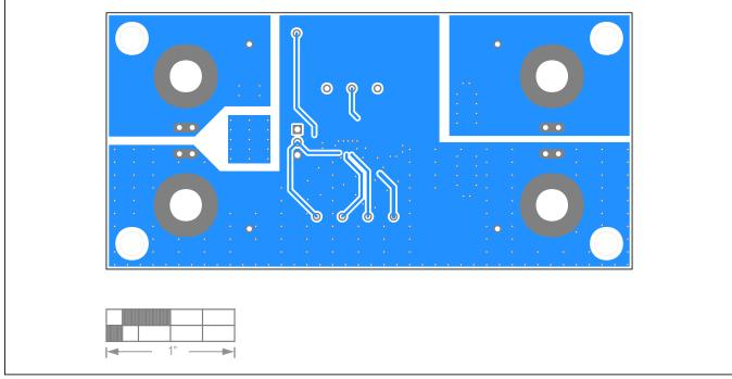
Figure 4. MAX16173 EV Kit PCB Layout—Bottom Side
