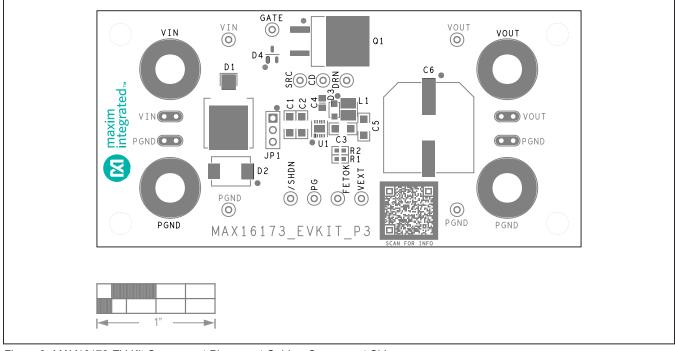
Figure 2. MAX16173 EV Kit Component Placement Guide—Component Side
