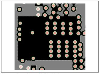
Figure 9. Second Layer (GND) with Keepout
