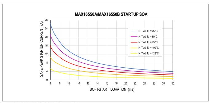
Figure 1. MAX16550A/MAX16550B Startup SOA
