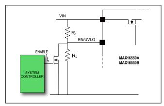
Figure 5. Programming Resistors for Input UVLO
