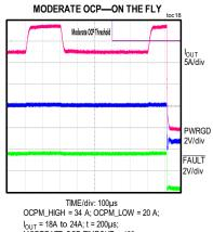
I<sub>OUT</sub> = 18A to 24A; t = 200μs; MODERATE OCP TIMEOUT = 100μs
