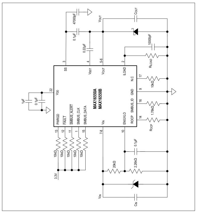
Figure 6. Reference Schematic
