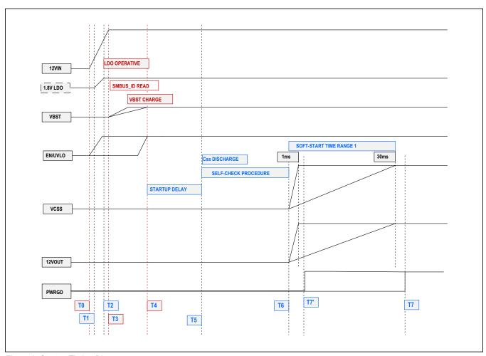
Figure 3. Startup Timing Diagram
