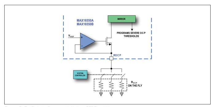
Figure 4. On-The-Fly Analog Programmable Moderate OCP Threshold
