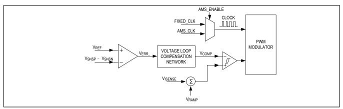
Figure 1. Simplified Control Architecture
