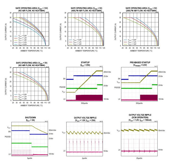
(Typical Application Circuit, tested on MAX16731EVKIT#,  $V_{DDH}$  = 12V,  $F_{SW}$  = 500kHz,  $T_A$  = +25°C, Inductor = FP1008R5-R220-R or 744309047 for  $V_{OUT}$  > 2.5V, unless otherwise noted.)
