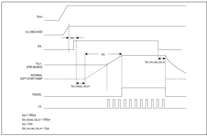
Figure 3. Startup and Shutdown Timing
