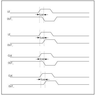
Figure 4. LE and CLK to OUT\_ Timing
