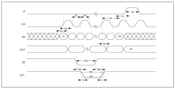
Figure 3. 4-Wire Serial-Interface Timing Diagram
