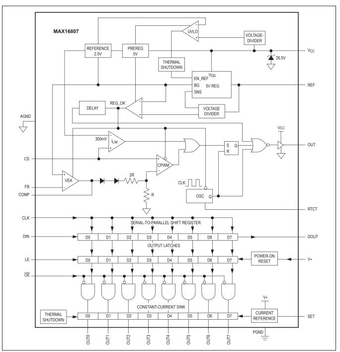
Figure 1a. Internal Block Diagram (MAX16807)
