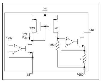
Figure 1b. OUT\_ Driver Internal Diagram
