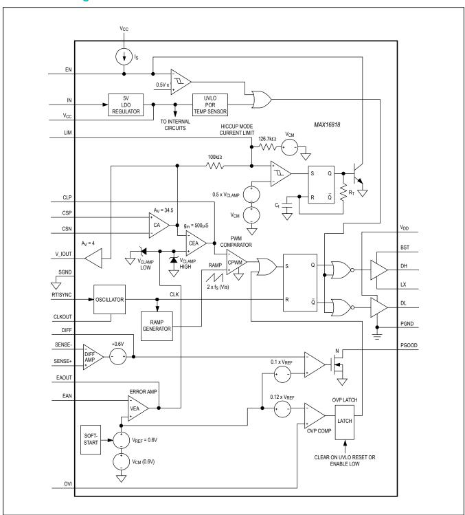
Figure 6. MAX16818 Functional Diagram
