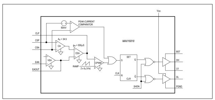
Figure 8. MAX16818 Phase Circuit
