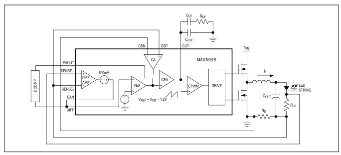
Figure 7. MAX16818 Control Loop
