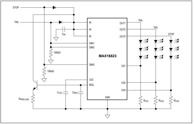
Figure 6. Preload Current Setting
