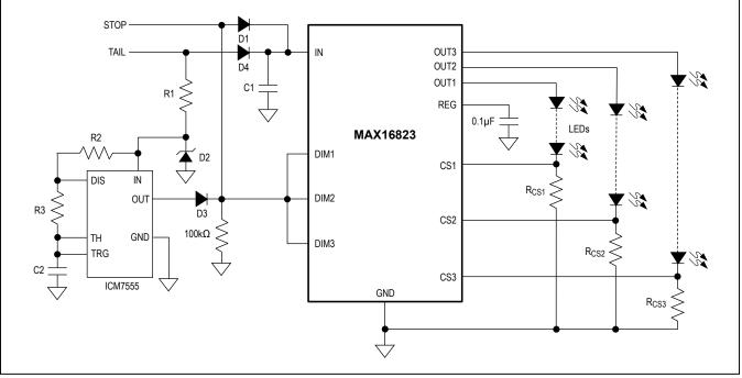
Figure 2. PWM Dimming Operation with ICM7555
