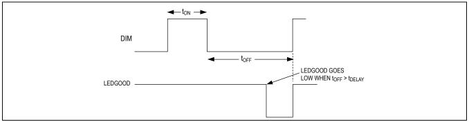
Figure 1. LEDGOOD Timing Delay
