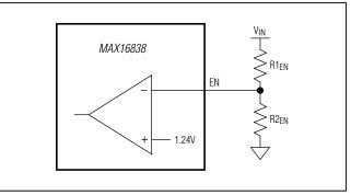
Figure 3. Setting the MAX16838 Undervoltage Lockout Threshold
