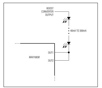
Figure 2. Configuration for Higher LED String Current
