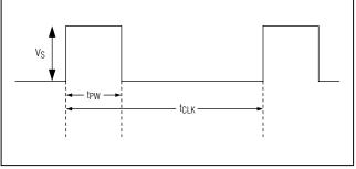
Figure 1. Synchronizing External Clock Signal
