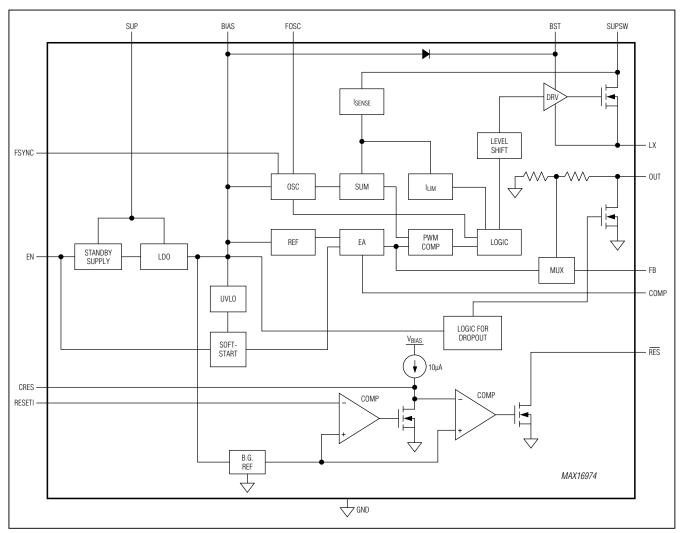
Figure 2. Internal Block Diagram
