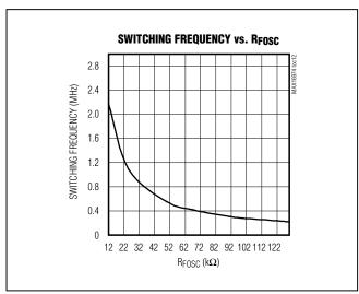
Figure 4. Switching Frequency vs. RFOSC
