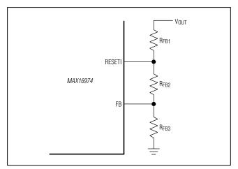
Figure 3. Output Voltage/Reset Threshold Resistive Divider Network
