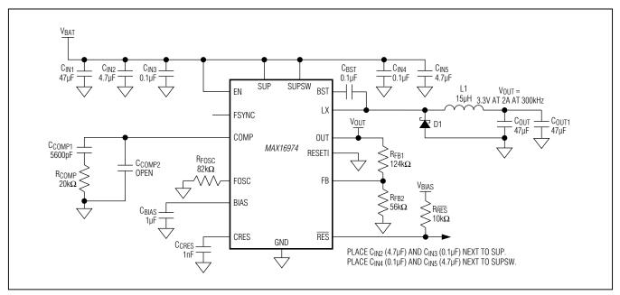
Figure 1. 3.3V Fixed Output Voltage Configuration
