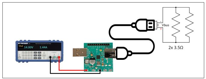
Figure 3: EV Kit Setup for Cable Compensation
