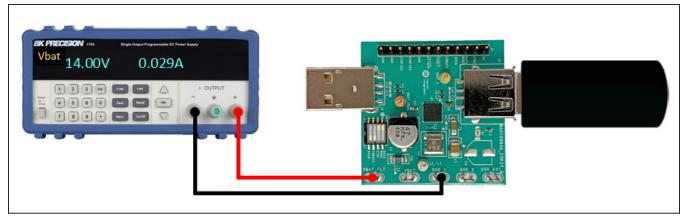
Figure 1: Initial EV Kit Setup
