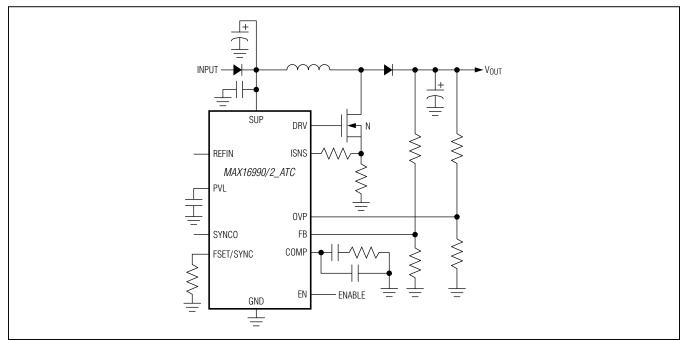
Figure 3. Application with Independent Output Overvoltage Protection
