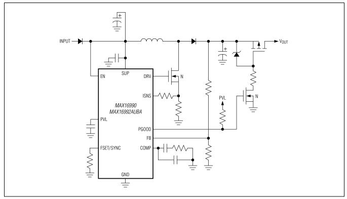
Figure 1. Application with Output Short-Circuit Protection
