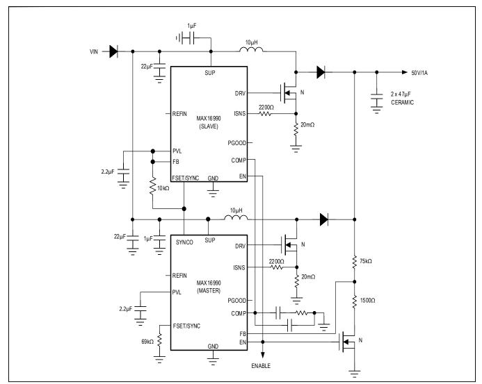
Figure 4. Two-Phase 400kHz Boost Application with Minimum Component Count
