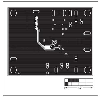
Figure 6. MAX16993 EV Kit PCB Layout—Solder Side
