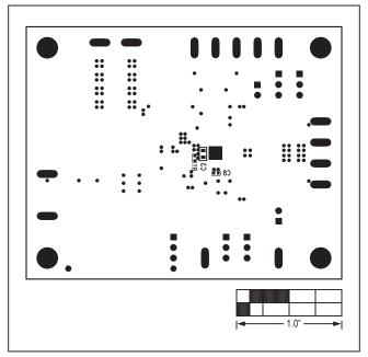
Figure 7. MAX16993 EV Kit Component Placement Guide—Solder Side
