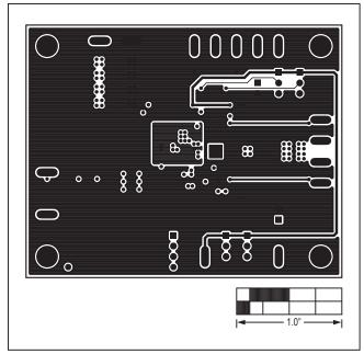
Figure 5. MAX16993 EV Kit PCB Layout—Layer 3
