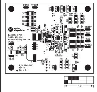
Figure 2. MAX16993 EV Kit Component Placement Guide—Component Side
