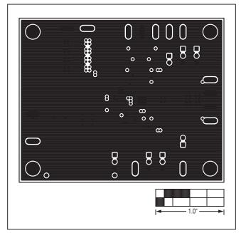
Figure 4. MAX16993 EV Kit PCB Layout—Layer 2
