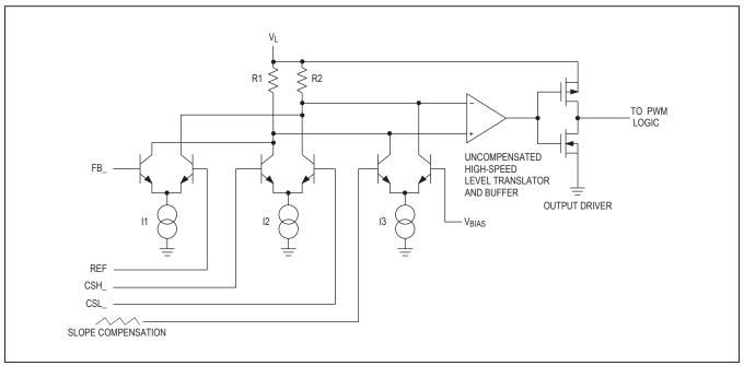
Figure 1. PWM Comparator Functional Diagram
