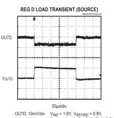
$V_{IND}$  = 1.8V,  $V_{REFIND}$  = 0.9V,  $C_{OUT}$  = 2 x 10 $\mu$ F, LOAD TRANSIENT I<sub>OUTD</sub>: 1A/div IS FROM 0 TO 1A SOURCING
