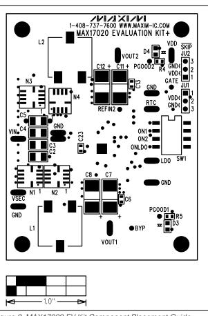
Figure 2. MAX17020 EV Kit Component Placement Guide— Component Side
