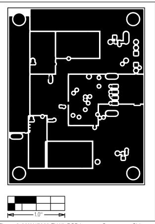
Figure 3. MAX17020 EV Kit PCB Layout—Component Side
