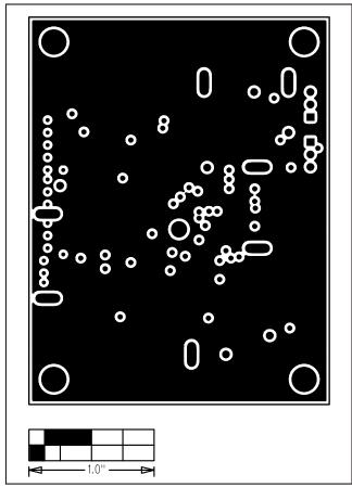
Figure 4. MAX17020 EV Kit PCB Layout—Layer 2 (PGND Plane)
