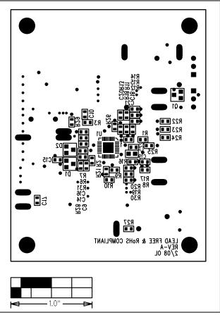
Figure 7. MAX17020 EV Kit Component Placement Guide— Solder Side
