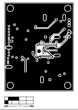
Figure 5. MAX17020 EV Kit PCB Layout—Layer 3 (PGND/Signal Layer)
