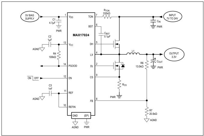
Figure 3. High Output-Voltage Application Using a Feedback Divider
