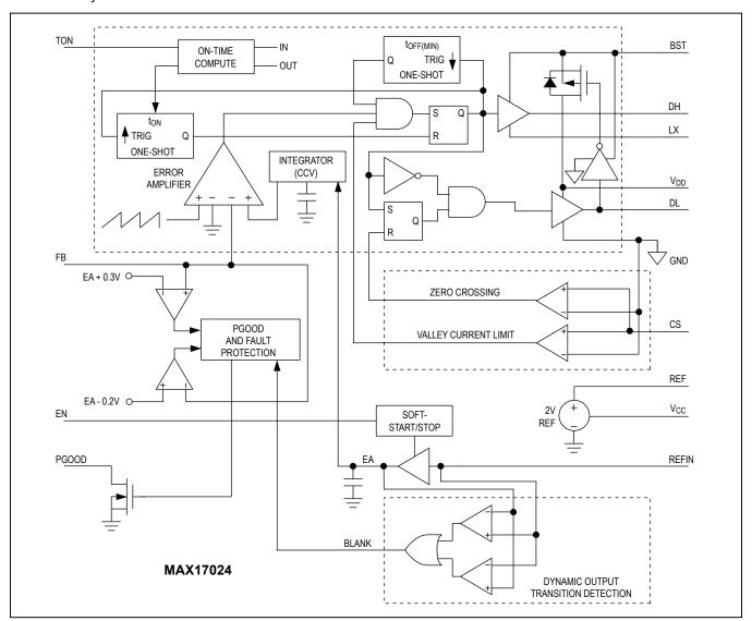
Figure 2. MAX17024 Functional Block Diagram
