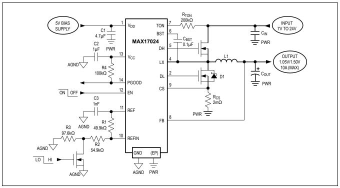
Figure 1. MAX17024 Standard Application Circuit
