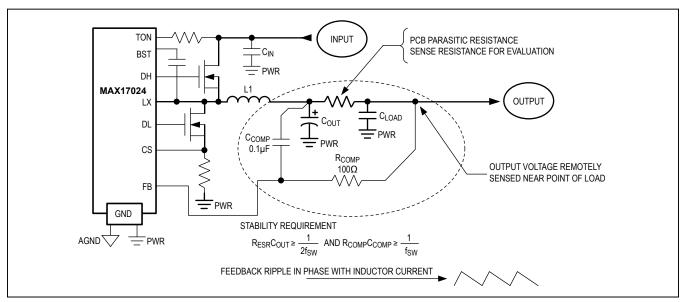
Figure 7. Remote-Sense Compensation for Stability and Noise Immunity
