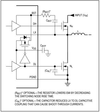
Figure 5. Gate Drive Circuit
