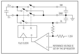
Figure 4. Negative Charge-Pump Regulator Block Diagram
