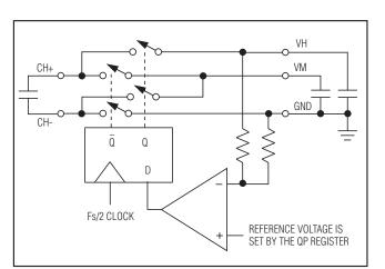
Figure 3. Positive Charge-Pump Regulator Control Block Diagram
