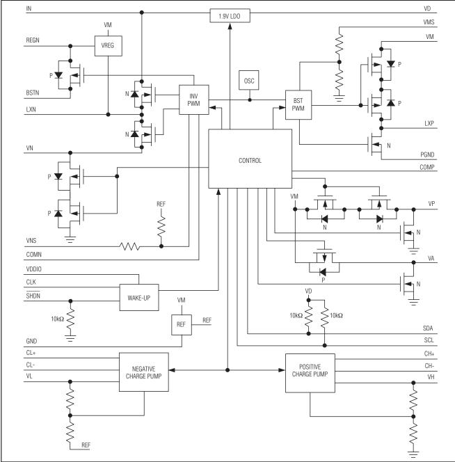
Figure 2. MAX17065 Functional Diagram
