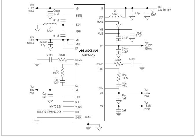
Figure 1. MAX17065 Typical Operating Circuit
