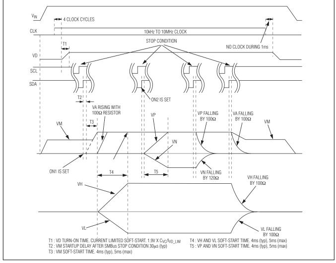
Figure 8. Startup and Shutdown Sequence
