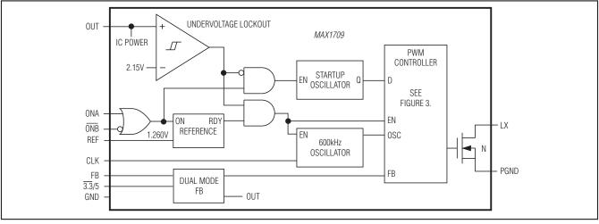
Figure 2. Simplified Functional Diagram
