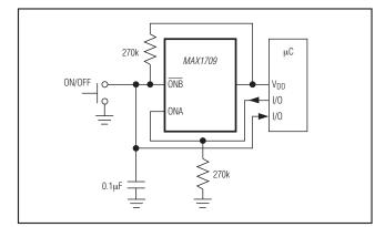
Figure 5. Momentary Pushbutton On-Off Switch
