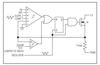
Figure 3. Simplified PWM Controller Functional Diagram
