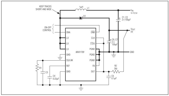
Figure 1. Standard Operating Circuit
