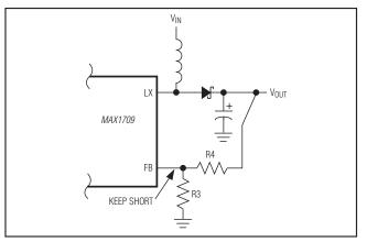
Figure 4. Adjustable Output Voltage
