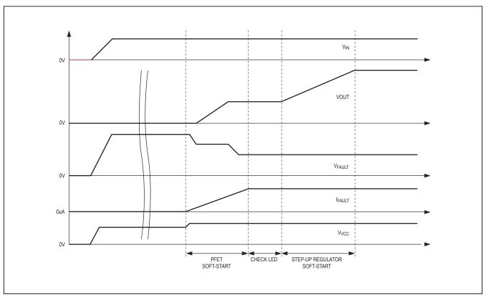
Figure 3. Startup Timing Sequence
