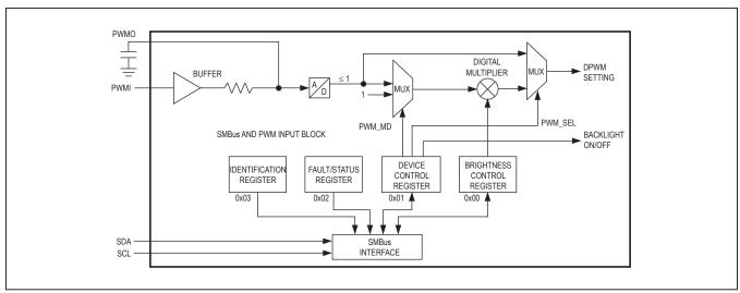
Figure 4. PWM and SMBus Interface Circuit
