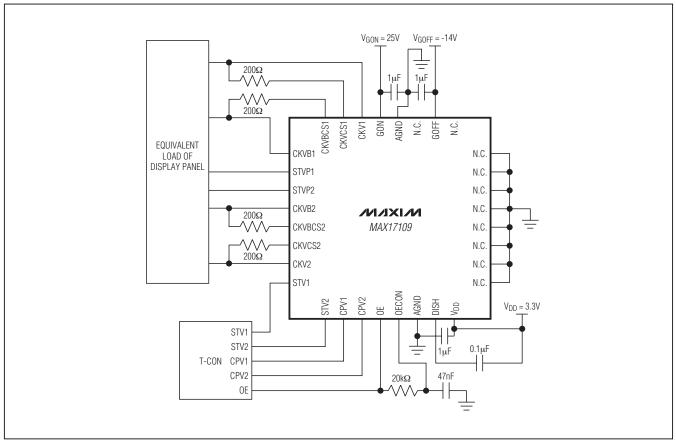
Figure 1. Typical Operating Circuit
