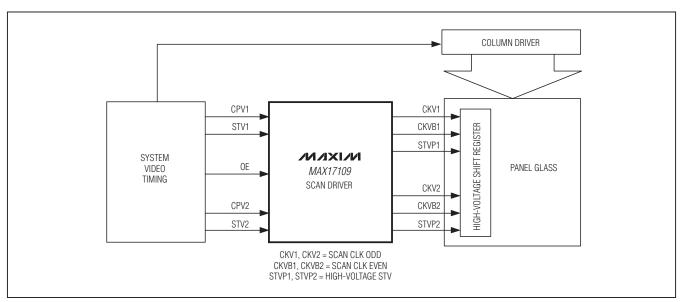
Figure 3. Scan Driver System Diagram
