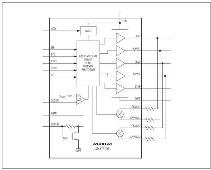
Figure 2. Functional Diagram
