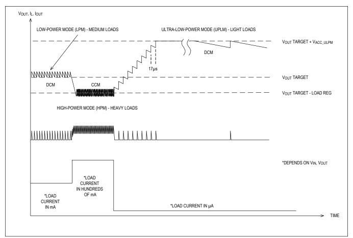
Figure 2. LPM, HPM, ULPM Transition Waveforms
