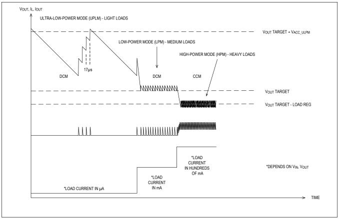
Figure 1. ULPM, LPM, HPM Transition Waveforms
