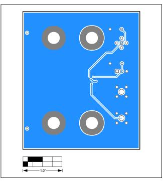
MAX17227J WLP EV PCB Layout Diagram—Bottom View
