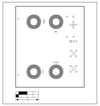
MAX17227J WLP EV PCB Layout Diagram—Bottom Silkscreen
