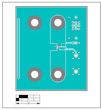
MAX17227J WLP EV PCB Layout Diagram—Top View
