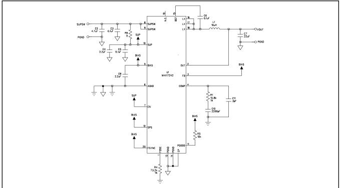
MAX17242 EV Minimal Component Schematic
