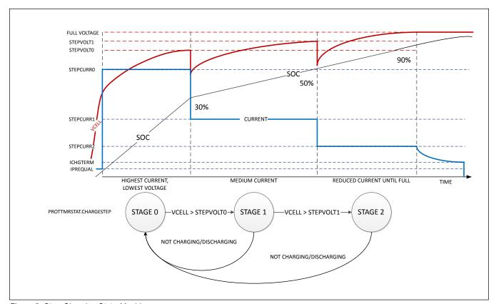
Figure 2. Step-Charging State Machine
