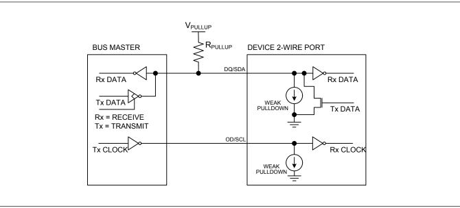
Figure 32. 2-Wire Bus Interface Circuitry
