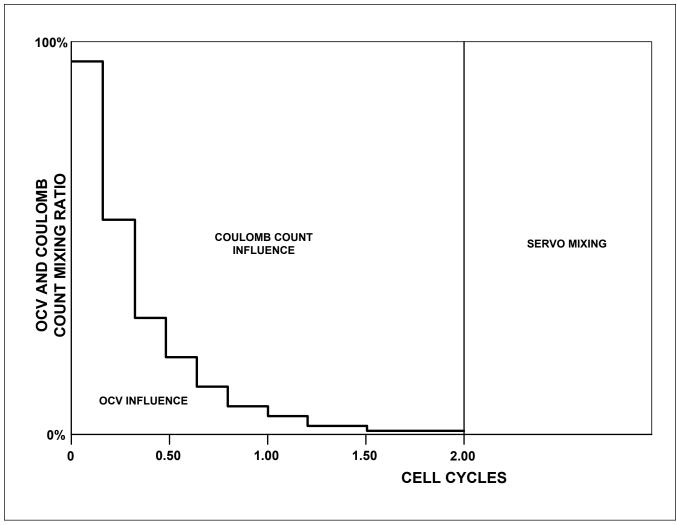
Figure 16. Voltage and Coulomb Count Mixing
