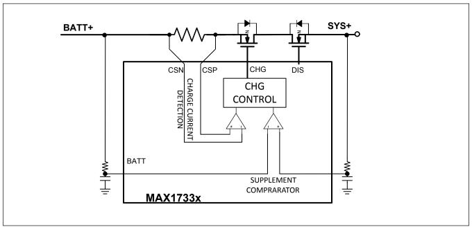
Figure 4. Supplement and Charging Comparators
