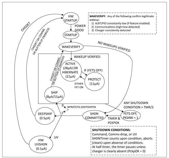
Figure 14. Power Mode Transition State Diagram
