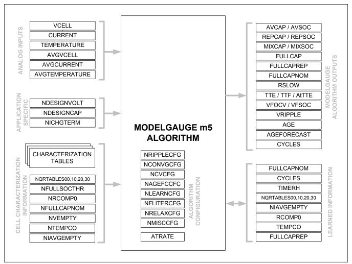
Figure 15. ModelGauge m5 EZ Registers
