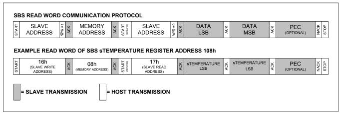
Figure 37. Example SBS Read Word Communication Sequence
