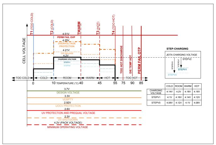
Figure 7. Programmable Voltage Thresholds
