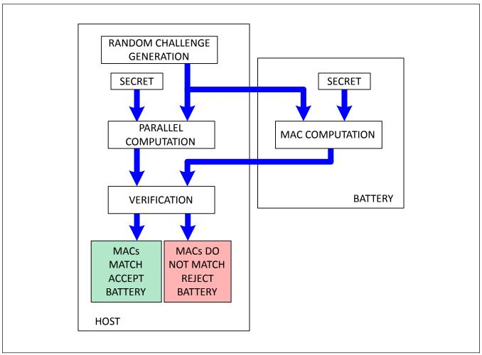
Figure 26. Procedure to Verify a Battery
