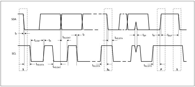
Figure 33. 2-Wire Bus Timing Diagram
