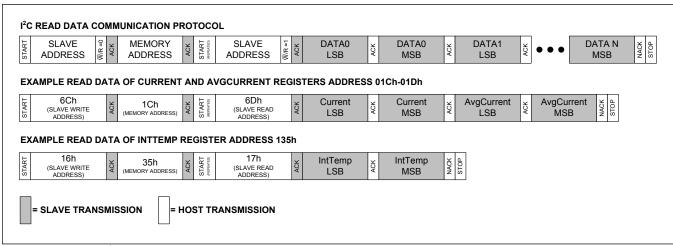
Figure 35. Example I<sup>2</sup>C Read Data Communication Sequence
