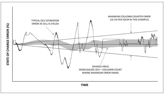
Figure 17. ModelGauge m5 EZ Typical Accuracy Example
