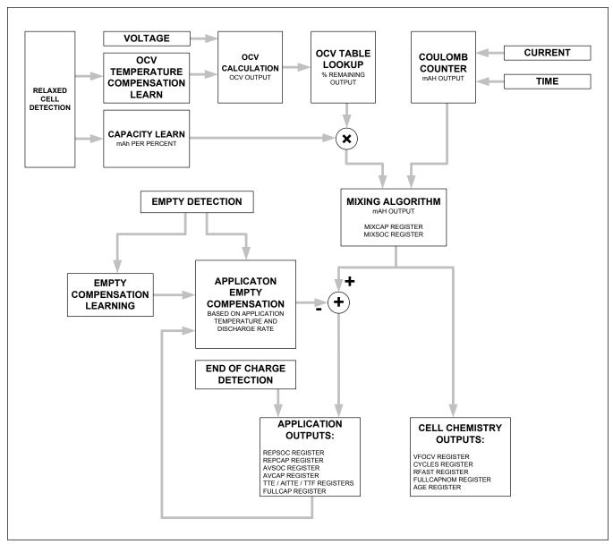
Figure 13. ModelGauge m5 EZ Block Diagram
