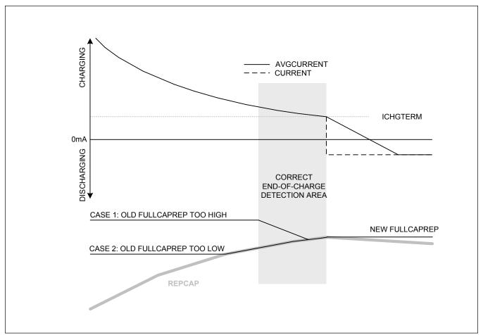
Figure 3. FullCapRep Learning at End-of-Charge
