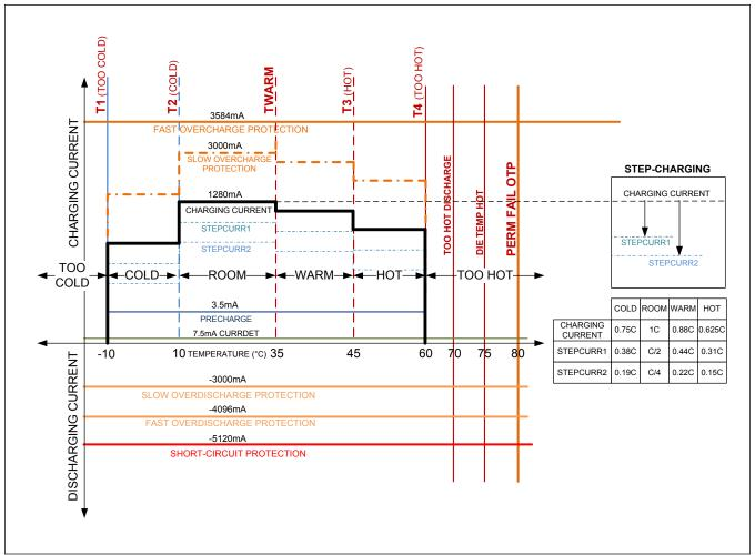
Figure 8. Programmable Current Thresholds
