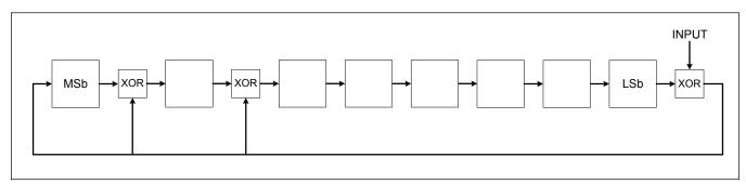
Figure 39. PEC CRC Generation Block Diagram
