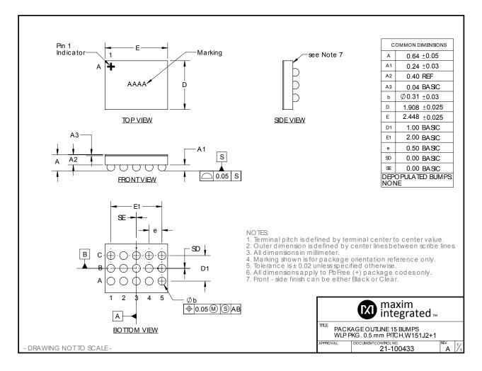
For the latest package outline information and land patterns (footprints), go to <a href="https://www.maximintegrated.com/packages">www.maximintegrated.com/packages</a>. Note that a "+", "#", or "-" in the package code indicates RoHS status only. Package drawings may show a different suffix character, but the drawing pertains to the package regardless of RoHS status.
