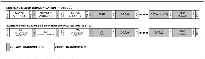
Figure 38. Example SBS Read Block Communication Sequence
