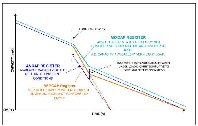
Figure 18. Handling Changes in Empty Calculation
