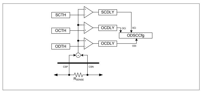
Figure 11. Overcurrent Comparator Diagram
