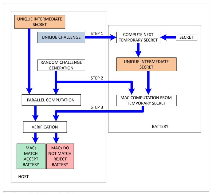
Figure 31. Procedure for 2-Stage Authentication
