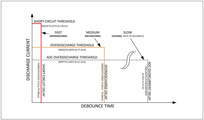
Figure 10. Fast, Medium, and Slow Overdischarge Protection
