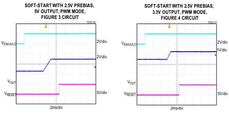
CONDITION: RESET IS PULLED UP TO VCC WITH A 10kQ RESISTOR CONDITION: RESET IS PULLED UP TO VCC WITH A 10kQ RESISTOR
