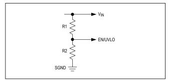
Figure 1. Setting the Input Undervoltage Lockout
