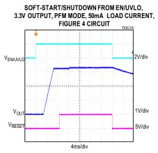
CONDITION:  $\overline{\text{RESET}}$  IS PULLED UP TO V<sub>CC</sub> WITH A 10k $\Omega$  RESISTOR
