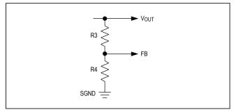
Figure 2. Setting the Output Voltage
