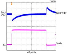
LOAD CURRENT STEPPED FROM 50mA TO 2.5A 3.3V OUTPUT, PFM MODE, FIGURE 4 CIRCUIT
