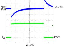
LOAD CURRENT STEPPED FROM 5mA TO 2.5A 5V OUTPUT, PFM MODE, FIGURE 3 CIRCUIT
