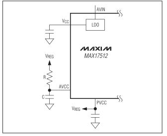
Figure 3. Configuring the MAX17512 to Use an External 5V Regulator (V\_{REG})
