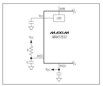
Figure 2. Configuring V<sub>CC</sub> to Power Control and Drive Circuitry
