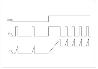
Figure 1. Modified Constant On-Time Valley Current-Control Scheme
