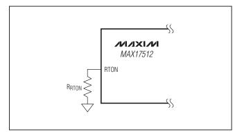
Figure 5. Programming the High-Side Switch On-Time
