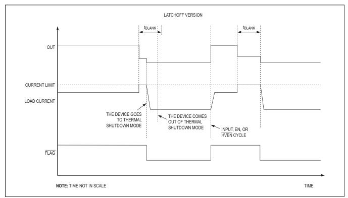
Figure 2. Latchoff Fault Diagram
