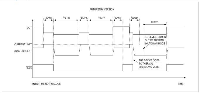
Figure 1. Autoretry Fault Diagram
