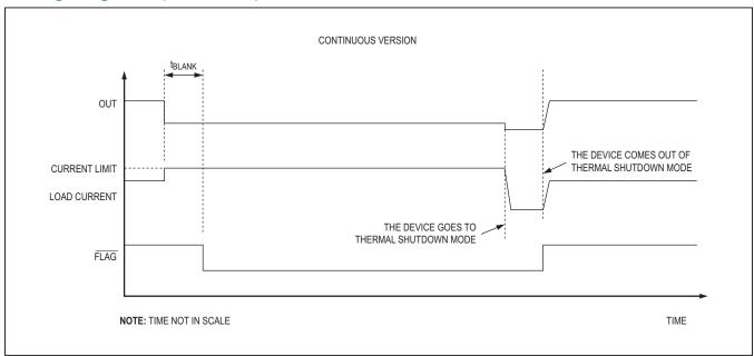
Figure 3. Continuous Fault Diagram
