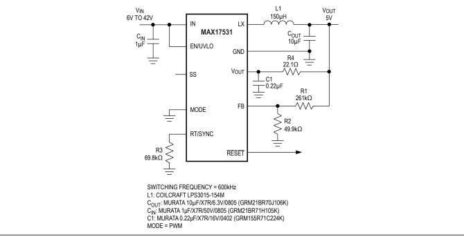
Figure 8. Small-Footprint 5V, 50mA Regulator
