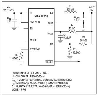
Figure 6. High-Efficiency 5V, 50mA Regulator
