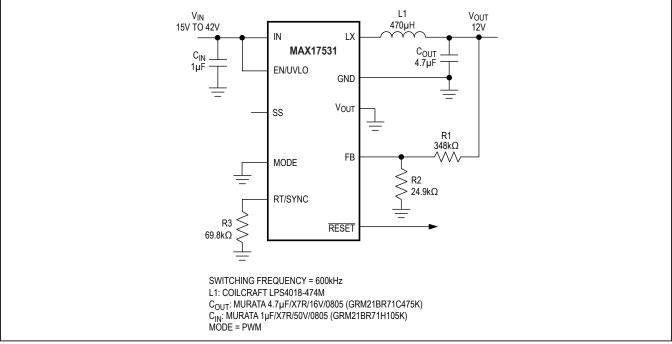
Figure 11. Small-Footprint 12V, 50mA Step-Down Regulator
