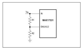
Figure 2. Adjustable EN/UVLO Network
