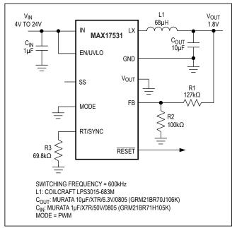
Figure 10. Small-Footprint 1.8V, 50mA Regulator
