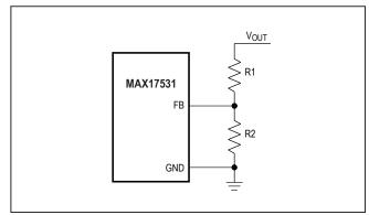
Figure 3. Setting the Output Voltage
