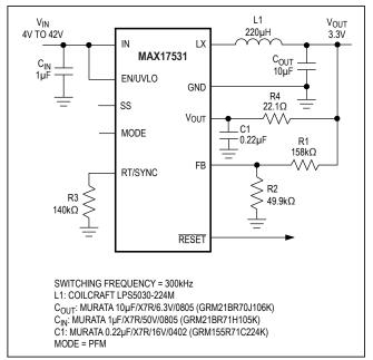
Figure 7. High-Efficiency 3.3V, 50mA Regulator
