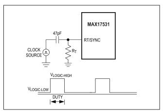
Figure 1. Synchronization to an External Clock
