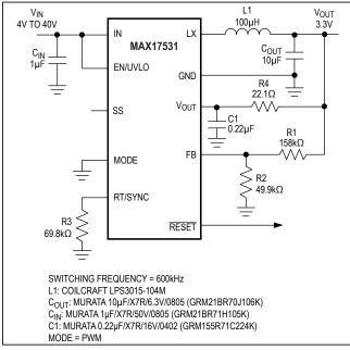
Figure 9. Small-Footprint 3.3V, 50mA Regulator
