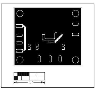
MAX17531 5V EV Kit (µMAX) PCB Layout—Solder Side
