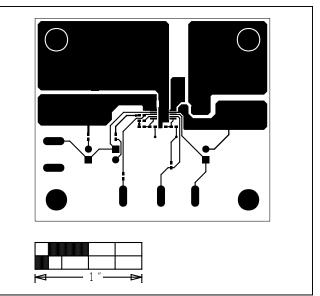
MAX17531 5V EV Kit (µMAX) PCB Layout—Component Side
