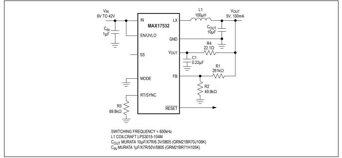
Figure 8. Small Footprint 5V, 100mA Regulator
