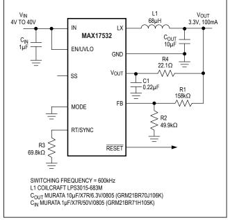
Figure 9. Small Footprint 3.3V, 100mA Regulator
