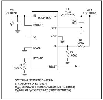
Figure 10. Small Footprint 1.8V, 100mA Regulator
