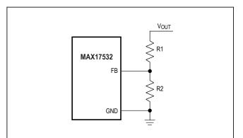
Figure 3. Setting the Output Voltage
