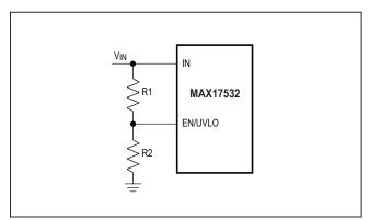
Figure 2. Adjustable EN/UVLO Network
