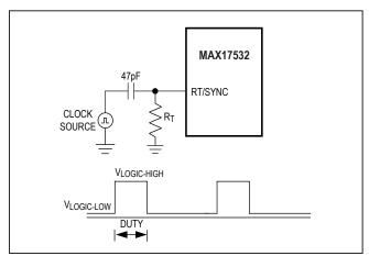
Figure 1. Synchronization to an External Clock
