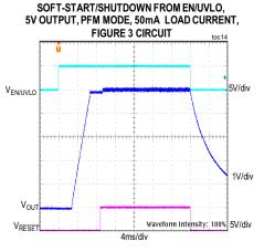
CONDITION:  $\overline{\text{RESET}}$  IS PULLED UP TO  $V_{CC}$  WITH A  $10k\Omega$  RESISTOR
