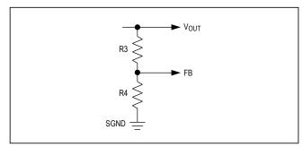
Figure 2. Setting the Output Voltage
