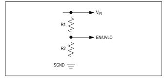
Figure 1. Setting the Input Undervoltage Lockout
