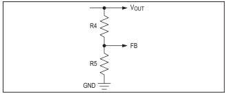
Figure 1. Setting the Output Voltage
