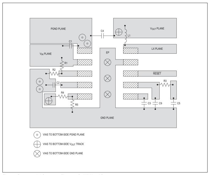
Figure 4. Recommended Component Placement for MAX17542G
