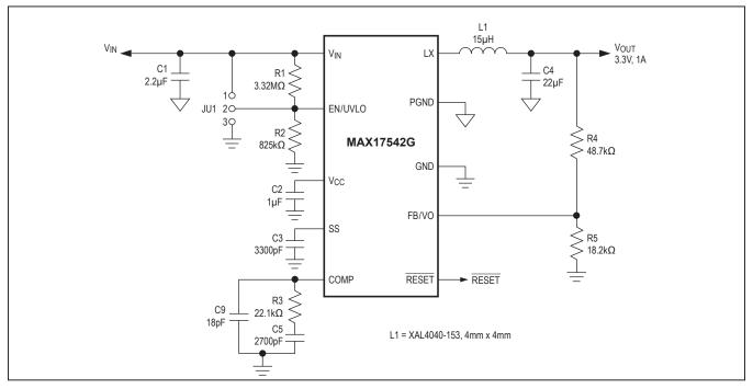
Figure 5. MAX17542G Application Circuit (3.3V Output, 1A Maximum Load Current)
