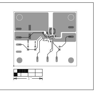
Figure 2. MAX17550 5V EV Kit (TDFN) PCB Layout— Component Side
