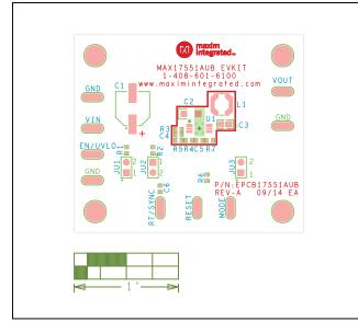
Figure 1. MAX17551 5V EV Kit (µMAX) Component Placement Guide—Component Side
