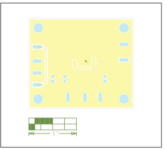
Figure 3. MAX17551 5V EV Kit (µMAX) PCB Layout—Solder Side
