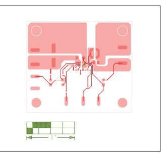
Figure 2. MAX17551 5V EV Kit (µMAX) PCB Layout— Component Side
