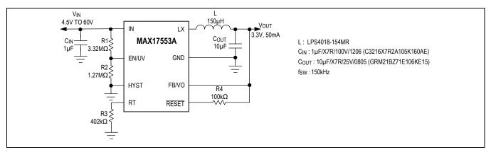
Figure 3. High-Efficiency 3.3V, 50mA Regulator
