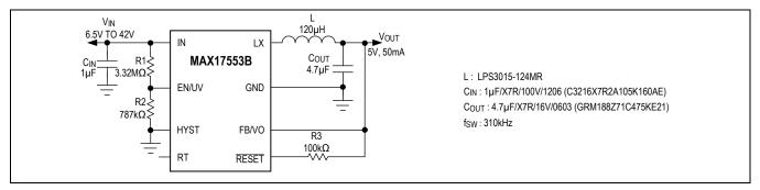
Figure 6. Small-Footprint 5V, 50mA Regulator
