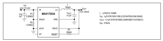
Figure 5. Small-Footprint 3.3V, 50mA Regulator
