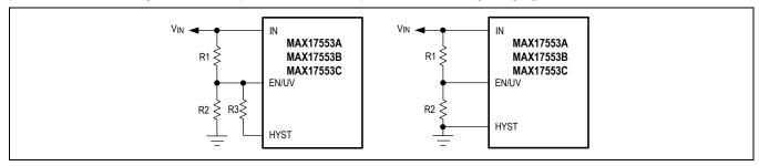
Figure 1. Setting the Input Undervoltage Level With and Without Hysteresis
