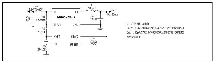
Figure 4. High-Efficiency 5V, 50mA Regulator
