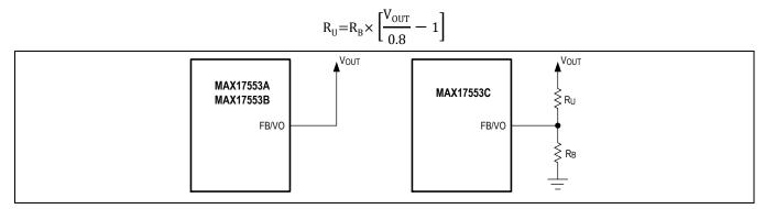
Figure 2. Setting the Output Voltage
